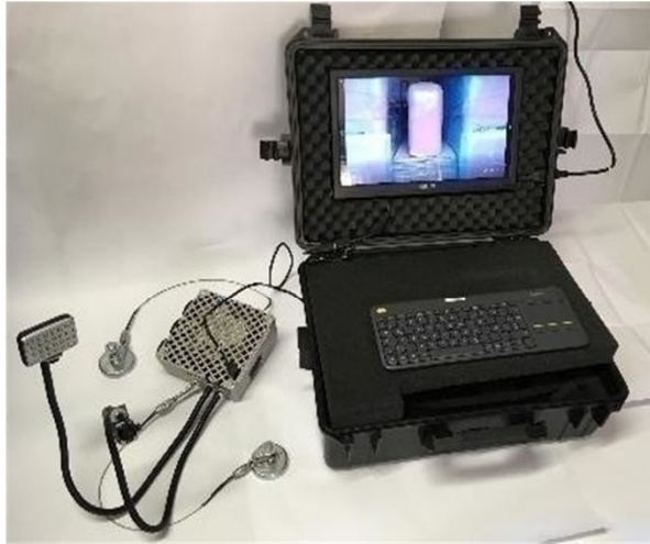
Buckling Visualisation System
