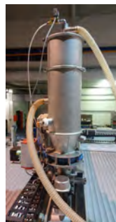
Figure 1(a). Extruder for automated feeding of the granules.
