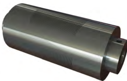
Figure 1. Schematic of a spreading roller with surface grooves for geometry-driven fiber spreading.
