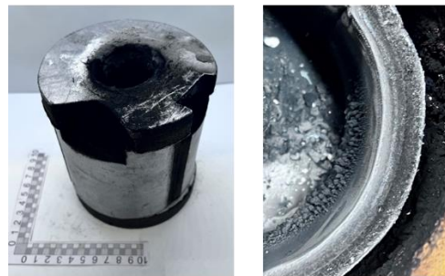
Fig 8. The reaction chamber after the pyrolysis test and the deposited CB on the inner surface.
