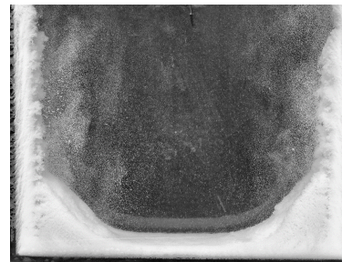
Fig.5. Stage 3: Swinging of turbulent snowing. The left and right areas of heavy turbulent snowing interact with each other. That started at around 6800 s and lasted till around 10000 s. During this stage, numerous avalanches occurred and the sedimentation in the corner region got quite steep.
