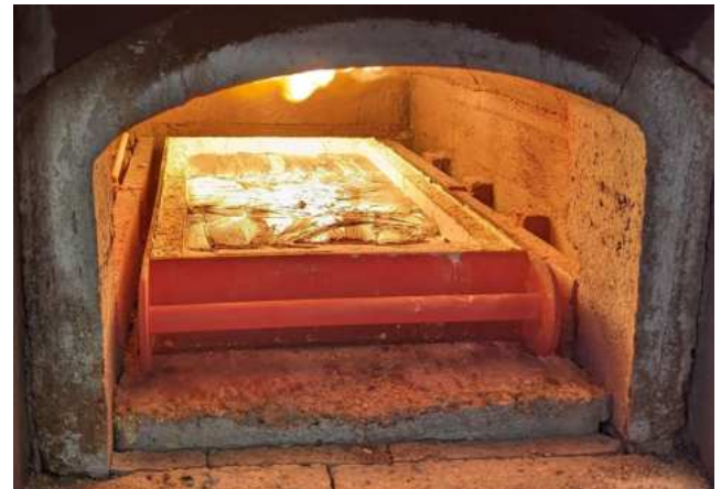
Fig. 2: Lab-scale hearth furnace for wrought alloys
