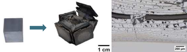
Fig. 3: CC sample before and after disintegration with zinc (left) and LOM image of the disintegration layer with the alternating layers of the Co-Zn phases and the carbide lamellae (right)
