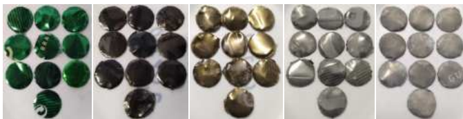
Fig. 1: Pictures of the aluminium platelets cut out from UBCs after pyrolysis; from left to right: original material, after 400 °C, after 450 °C, after 500 °C, after 550 °C
