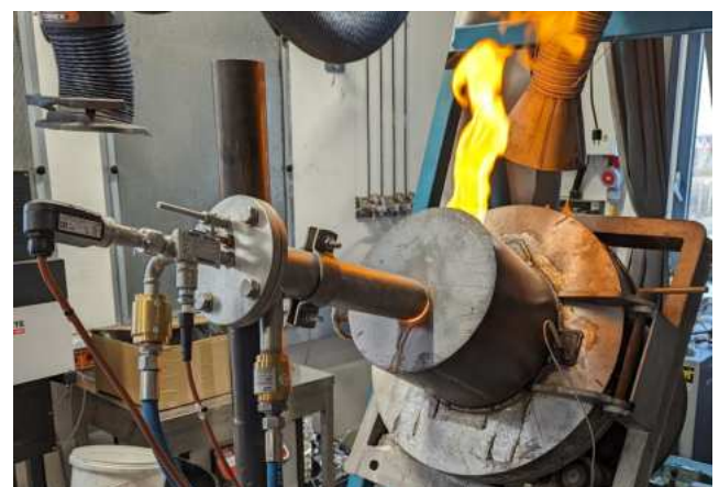
Fig. 3: Lab-scale tilting drum furnace for cast alloys
