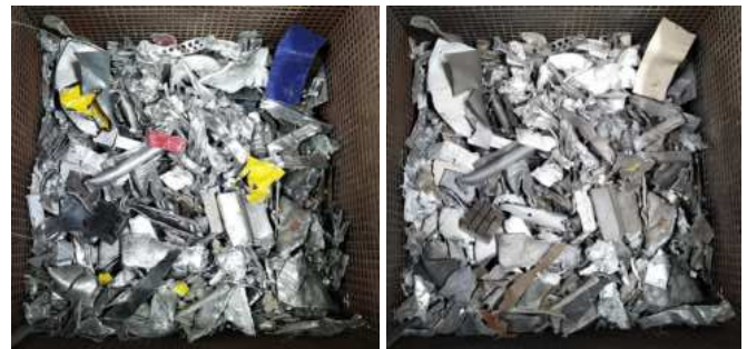
Fig. 2: Industrial scrap before (left) and after (right) pyrolysis at 550 °C for 6 h
