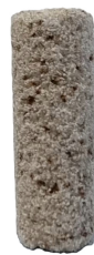
Typical Micro-CT Sample of a Berea Sandstone with a diameter of 4 mm
