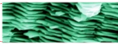
Fig. 3: Step-wise fracture of layered nacre
