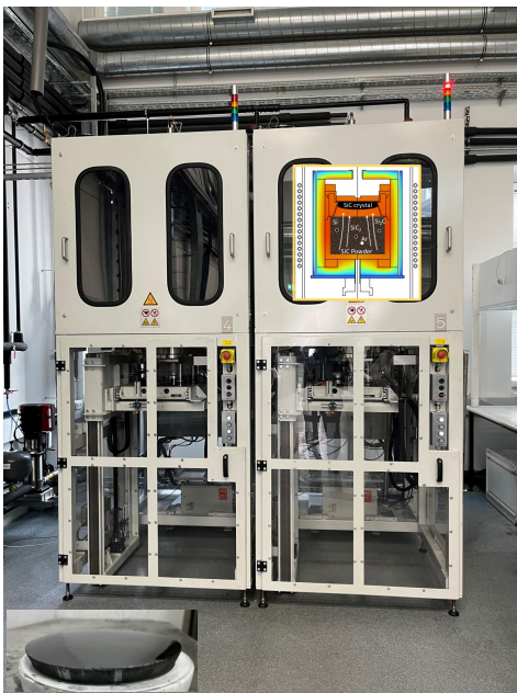
Single crystals of SiC are grown in furnaces with the physical vapor transport (PVT) method. A schematic is shown in the window of the right furnace. An example of an obtained single crystal boule is shown on the bottom left.
