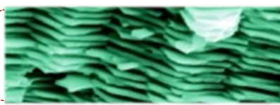
Fig. 3: Step-wise fracture of layered nacre
