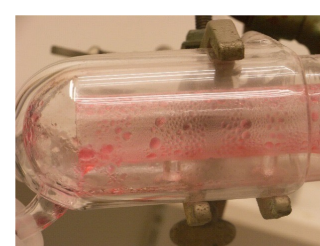
Fig. 18 Zones of droplet impact nebulizing a methylene red solution
